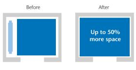
The KONE NanoSpace uses ultra-compact balancing weights, leaving more space for a larger car with no changes to the shaft.
